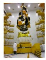
THE UPPER COMPOSITE INTEGRATION FACILITY (UCIF) Spacecraft mating with the Fregat upper stage is performed in this 587 sq. meter high bay, along with fairing encapsulation. The facility has equipment and personnel airlocks and an on-site control room. The remote control room in the customer office area can also be used to monitor activities in the UCIF. The data network allows the customer to carry out spacecraft testing via direct links with EGSE installed in the PPF control room.
