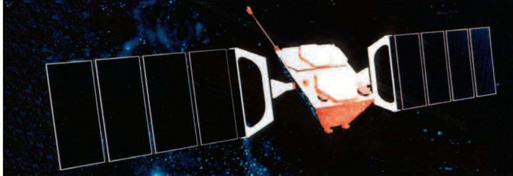
Each first-generation Globalstar satellite, designed by Space Systems/Loral, is a three-axis stabilized spacecraft consisting of a trapezoidal main body, two solar arrays, and a boom-mounted magnetometer. Mass of the satellite is approximately 450 kilograms.
