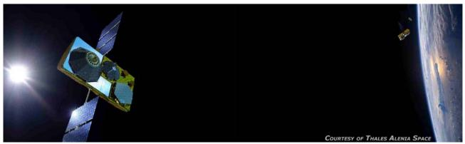
The new Globalstar second-generation low-earth-orbit (LEO) satellite is a three-axis stabilized spacecraft consisting of a trapezoidal main body with two solar arrays. In 2006 Globalstar contracted Thales Alenia Space for the design, manufacture and delivery of its second-generation constellation satellites. The first six satellites being launched were delivered to Globalstar in August of this year.
