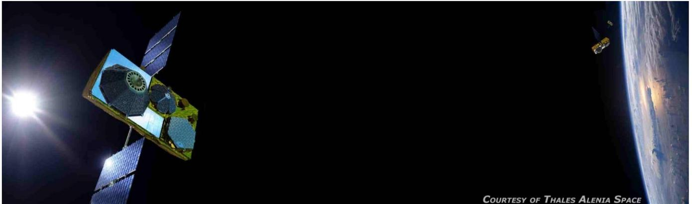
The new Globalstar second-generation low-earth-orbit (LEO) satellite is a three-axis stabilized spacecraft consisting of a trapezoidal main body with two solar arrays. In 2006 Globalstar contracted Thales Alenia Space for the design, manufacture and delivery of its second-generation constellation satellites. The first six satellites being launched were delivered to Globalstar in August of this year.
